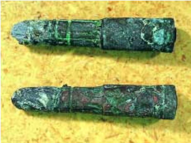
Bullets showing copper and lead alloy corrosion products.
