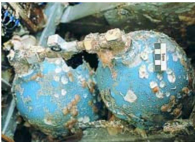
Aluminium cylinders showing the effects of attack by chloride ions.
