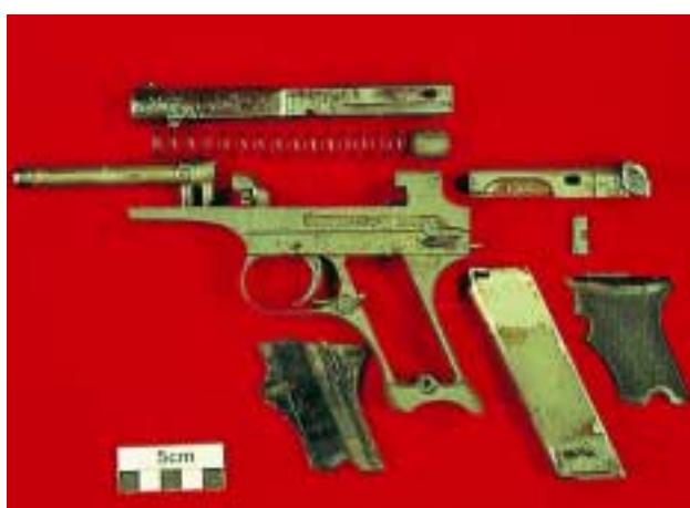
Pistol after treatment with citric acid/heat, fish oil/white spirit solution.
